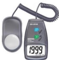
Figure 4: KM-99 digital lux meter used to measure PIT value and surface reflectance.
