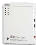
Figure 4: HOBO data loggers used for long-term monitoring
